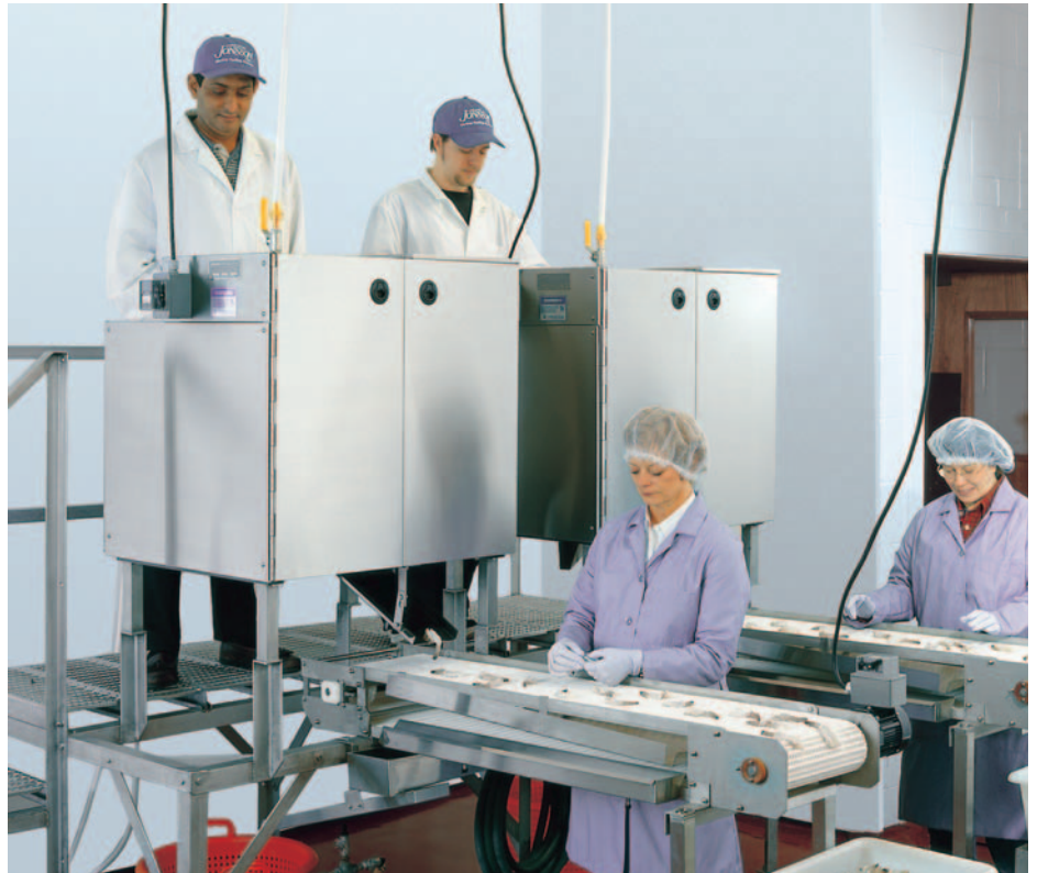
Water Conservation Peeling Systems, such as the two-station system pictured above, use 50 to 70% less water than Standard Systems.
